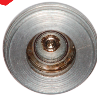
Push-button was abraded due to incorrect use
