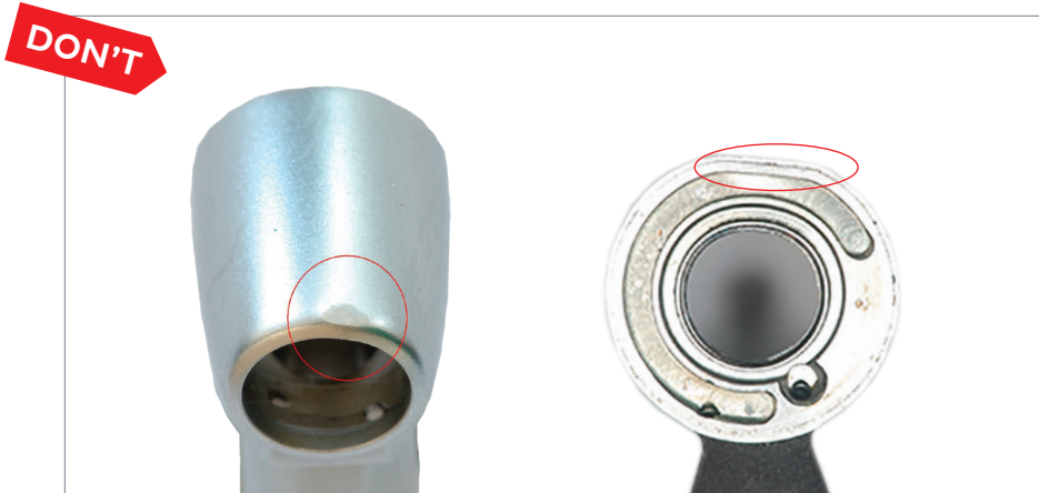
Handpiece showing damage from being dropped
